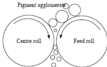
Figure 1 - Pigment Particles entering a three roll mill
